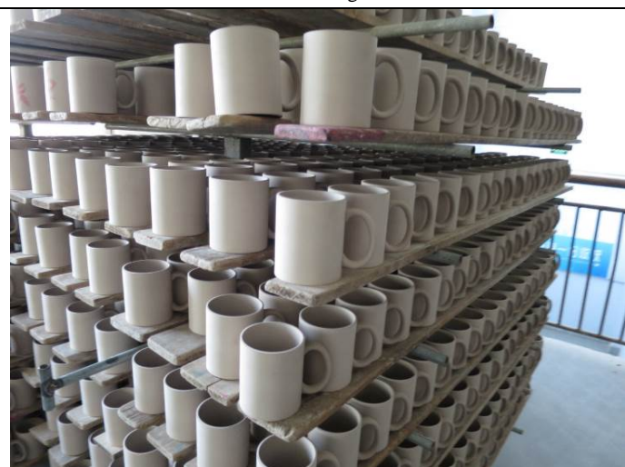
Ready for glazing
