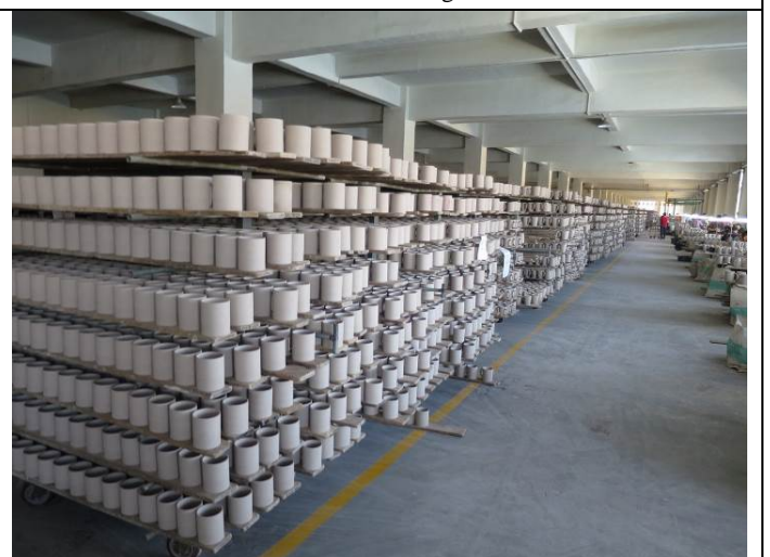
Ready for glazing
